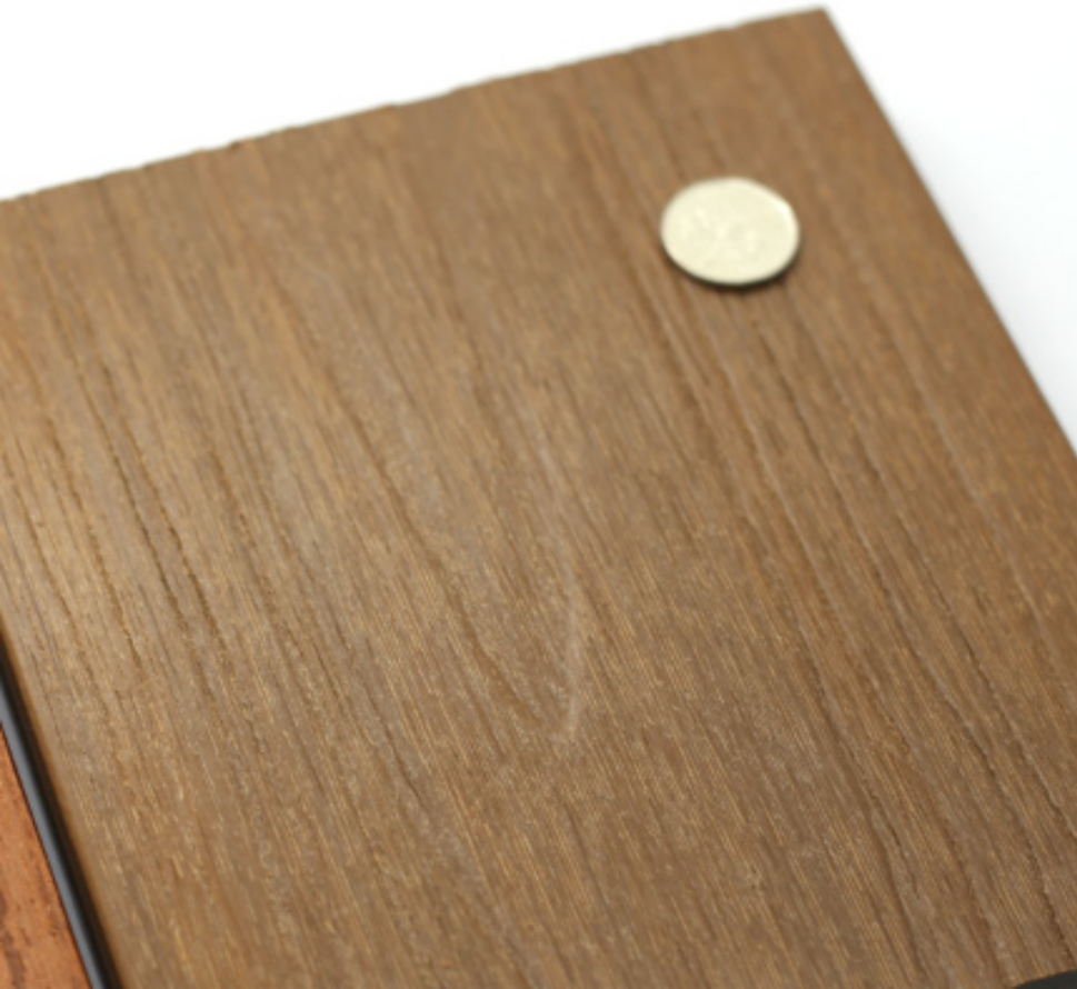
UltraShield decking Insignificant marks
