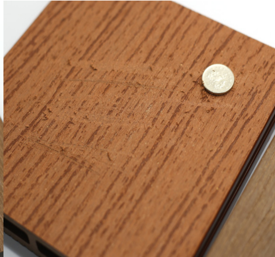
Conventional decking Significant marks & material worn off
